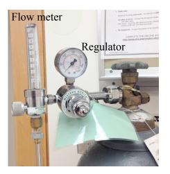
A flow meter measures the volume of gas passing thru the nozzle per unit of time. Generally, the flow meter will measure the amount of CO2 in liters per minute.
